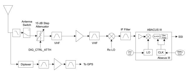
Figure 3-2. Receiver Block Diagram (VHF)
