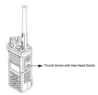
Figure 8-49. Securing the Cover
