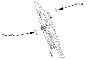
Figure 8-25. Serviceable Components – Main Board Assembly
