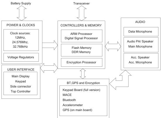
Figure 3-11. Controller Block Diagram
