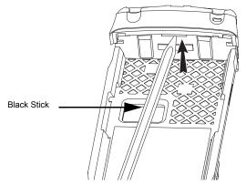
Figure 8-17. Disengage the Shroud
