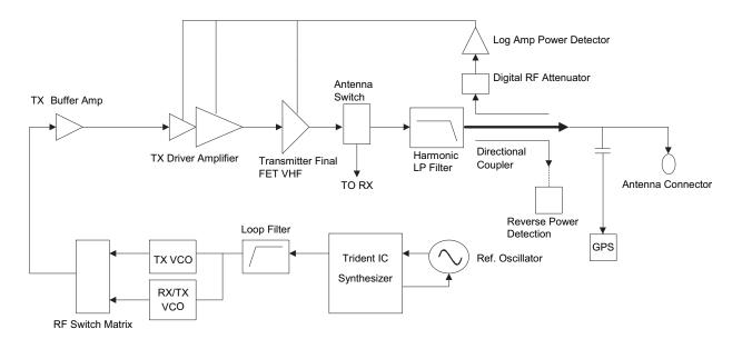
Figure 3-7. Transmitter (VHF) Block Diagram
