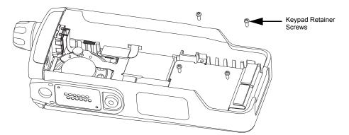
Figure 7-16. Remove the Keypad Retainer Screws
