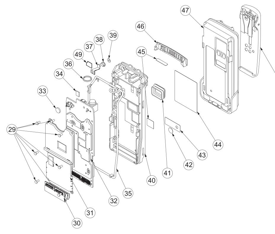
Exploded Views and Parts Lists: APX 1000 Back Kit Exploded View
