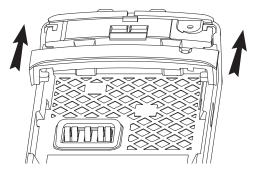
Figure 7-33. Assemble the Shroud
