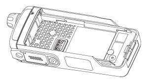
Figure 7-40. Assemble the Vacuum Port Seal
