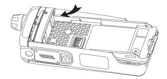
Figure 7-36. Slide chassis assembly into Front Housing
