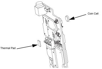
Figure 8-22. Serviceable Components – Main Board Assembly
