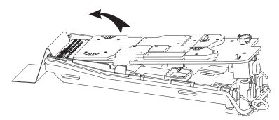
Figure 7-12. Lift up the Main Board from the Chassis
