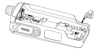
Figure 7-17. Detach the Keypad Flex from Keypad Board
