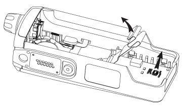
Figure 7-18. Remove the Keypad Board
