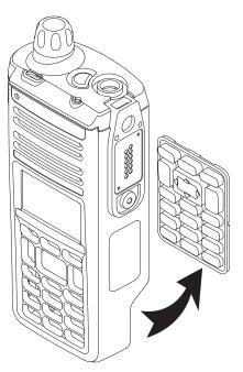
Figure 8-21. Remove the Keypad
