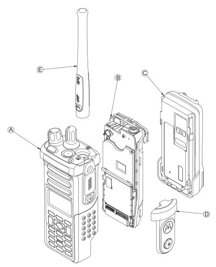
Figure 8-1. APX 2000/ APX 4000 (Two Knobs) Partial Exploded View
