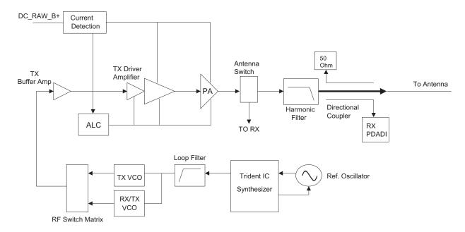
Figure 3-6. Transmitter Block Diagram
