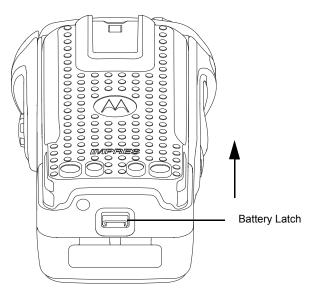
Figure 8-2. Lifting up the latch
