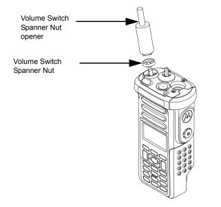
Figure 8-9. Removing the Volume Switch Spanner Nut
