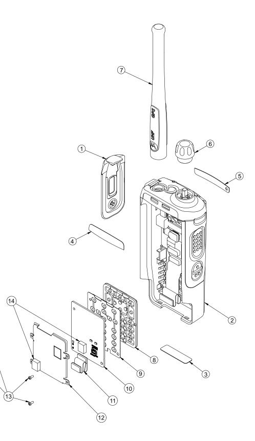
Figure 9-1. APX 1000 Front Kit Exploded View
