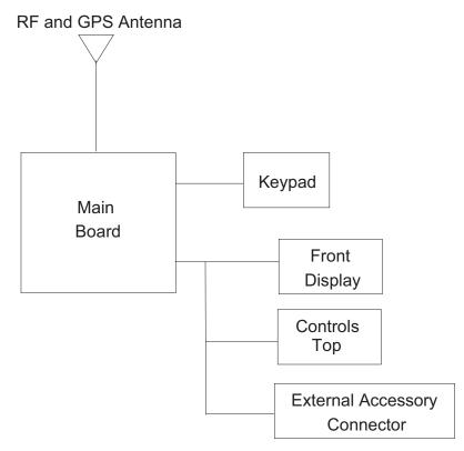
Figure 3-1. APX 1000 Overall Block Diagram
