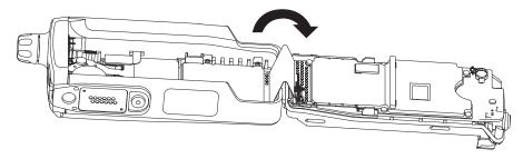
Figure 8-8. Remove the Chassis Assembly
