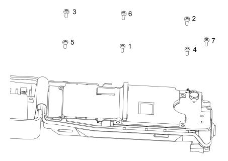
Figure 8-36. Torque in the Chassis Screws\
