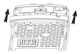
Figure 8-35. Assemble the Shroud
