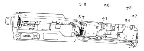
Figure 7-32. Torque in the Keypad Retainer Screws
