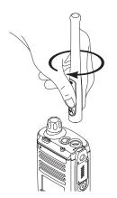
Figure 7-39. Attaching the Antenna
