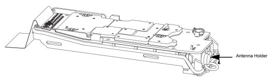
Figure 8-14. Remove the Main O-Ring at the antenna holder
