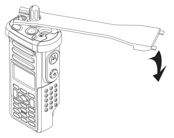
Figure 8-30. Servicing the Channel Knob
