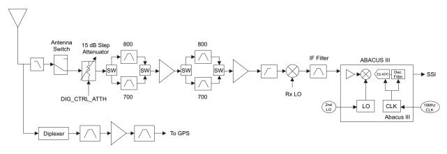
Figure 3-4. Receiver Block Diagram (700/800 MHz)
