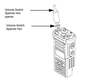
Figure 8-46. Tighten the Volume Switch Spanner Nut
