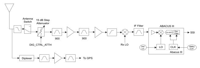
Figure 3-5. Receiver Block Diagram (900 MHz)
