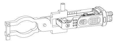
Figure 8-56. Attaching Pressure Test Fixture
