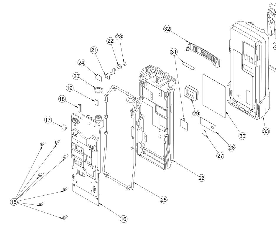
Figure 9-2. APX 1000 Back Kit Exploded View
