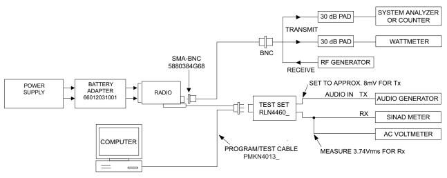
Figure 6-1. Radio Alignment Test Setup
