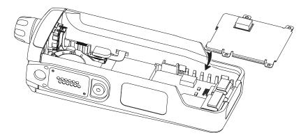
Figure 7-28. Place Keypad Retainer over the Keypad Board
