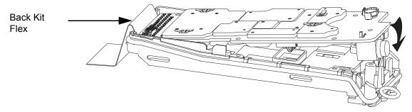
Figure 8-33. Assemble the RF Board
