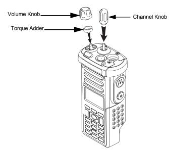
Figure 8-47. Reassemble the Volume Knob and Channel Knob
