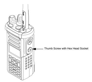
Figure 8-7. Removing the Thumb Screw
