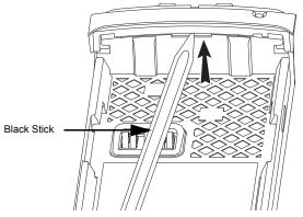
Figure 8-14. Disengage the Shroud
