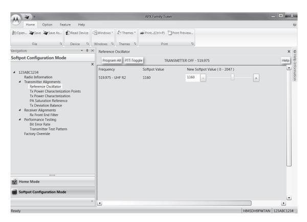
Figure 6-7. Reference Oscillator Alignment Screen (UHF2)
