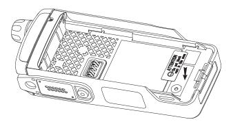
Figure 7-41. Assemble the Ventilation Label
