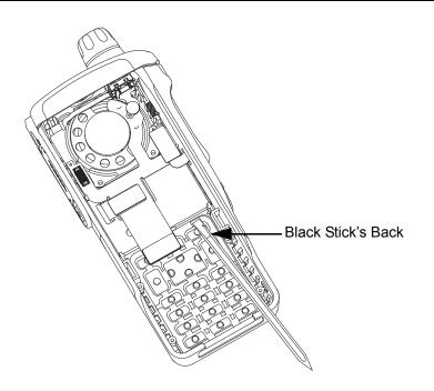
Figure 8-30. Assemble the Keypad
