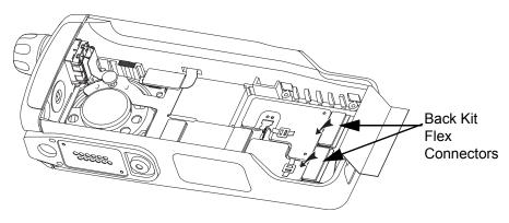
Figure 7-32. Plug in the Back Kit Flex Connectors
