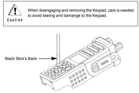
Figure 8-23. Disengage the Keypad
