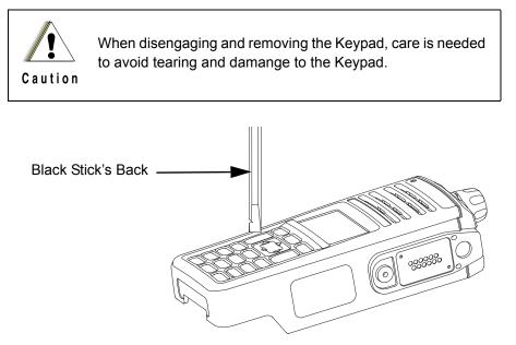
Figure 7-20. Disengage the Keypad
