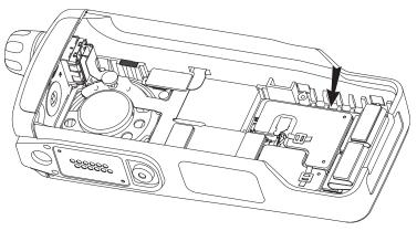
Figure 7-19. Remove the Keypad Board
