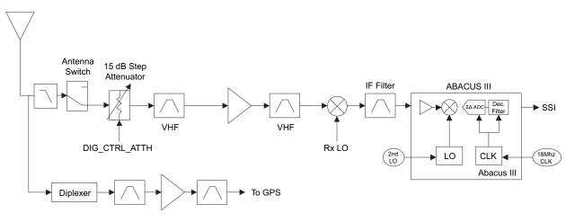
Figure 3-2. Receiver Block Diagram (VHF)
