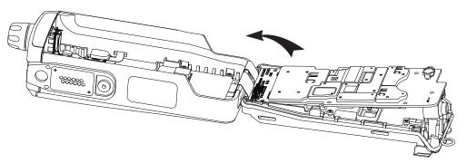
Figure 7-11. Lift up the Main Board from the Chassis
