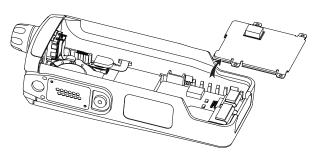
Figure 7-16. Remove the Keypad Retainer
