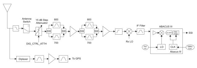
Figure 3-4. Receiver Block Diagram (700/800 MHz)
