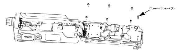
Figure 7-9. Remove the chassis screws
