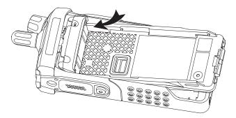
Figure 8-43. Slide chassis assembly into Front Housing
