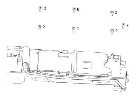
Figure 8-12. Remove the Chassis Screws
