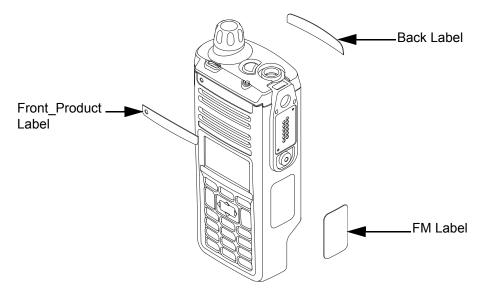
Figure 8-24. Serviceable Components – Main Housing
