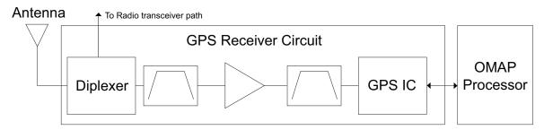
Figure 3-3. GPS Diagram
