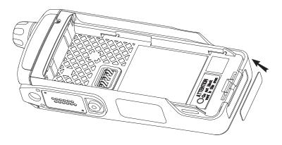
Figure 7-42. Assemble the Bottom Label
