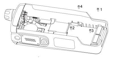
Figure 7-34. Torque in the Keypad Retainer Screws
