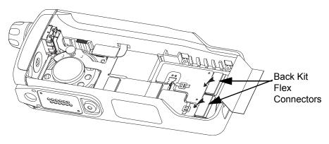
Figure 8-32. Plug in the Back Kit Flex Connectors
