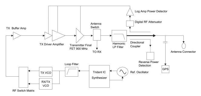
Figure 3-4. Transmitter (900 MHz) Block Diagram
