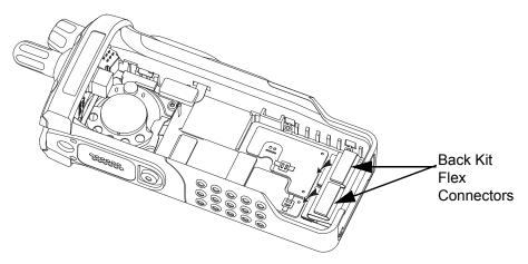
Figure 8-39. Plug in the Back Kit Flex Connectors
