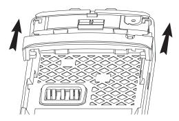
Figure 7-35. Assemble the Shroud
