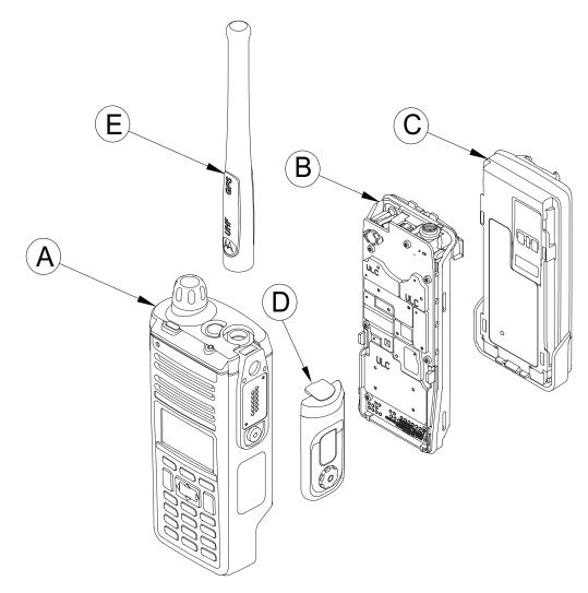
Figure 7-1. APX 1000 Partial Exploded View
