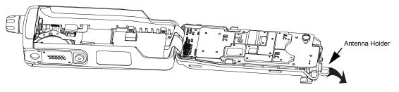
Figure 7-10. Remove the Main O-Ring at the antenna holder
