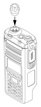
Figure 7-38. Reassemble the Multi Function Knob
