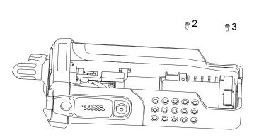
Figure 8-41. Torque in the Keypad Retainer Screws
