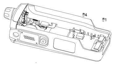
Figure 7-29. Torque in the Keypad Retainer Screws
