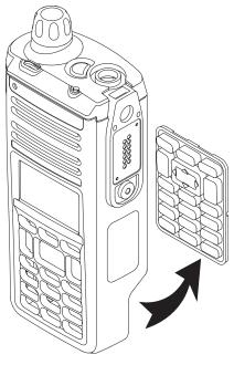
Figure 7-20. Remove the Keypad
