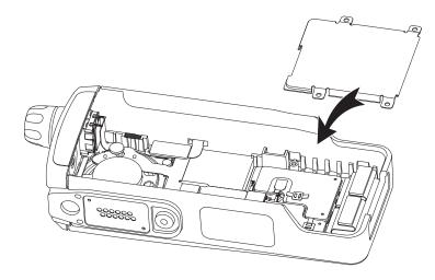
Figure 7-33. Place Keypad Retainer over the Keypad Board
