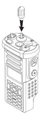
Figure 8-31. Align D-shaped part of the shaft with the D-shaped hole
