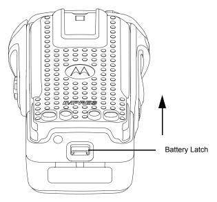
Figure 7-2. Lifting up the latch
