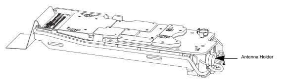
Figure 8-11. Remove the Main O-Ring at the antenna holder
