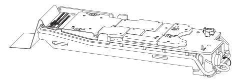
Figure 8-27. Assemble the Main O-Ring at Antenna Holder
