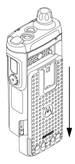
Figure 7-3. Removing the Battery
