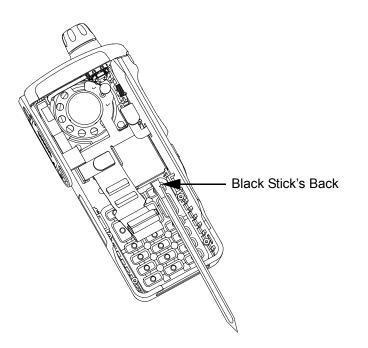
Figure 7-25. Assemble the Keypad
