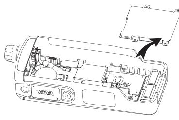
Figure 8-17. Remove the Keypad Retainer
