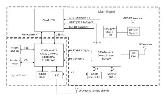
Figure 3-10. GPS/Bluetooth/Accelerometer Block Diagram
