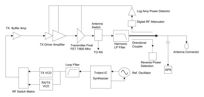
Figure 3-8. Transmitter (700/800 MHz) Block Diagram
