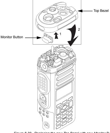
Figure 8-32. Replacing the new Top Bezel with new Monitor Button
