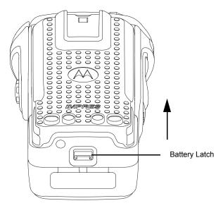
Figure 7-2. Lifting up the battery latch
