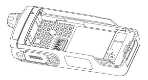
Figure 7-42. Assemble the Vacuum Port Seal
