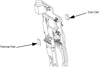
Figure 7-22. Serviceable Components – Main Board Assembly
