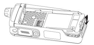
Figure 7-37. Assemble Back Kit and Front Kit together
