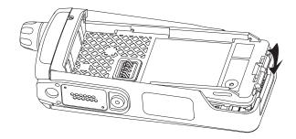
Figure 7-35. Assemble Back Kit and Front Kit together
