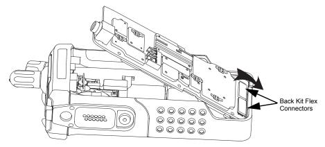
Figure 8-16. Unplug the Back Kit Flex connectors
