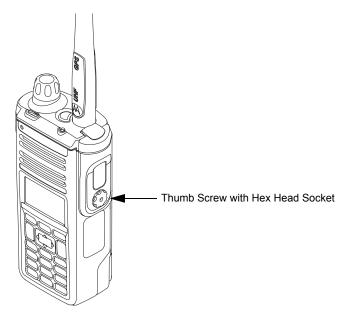
Figure 7-39. Securing the Cover
