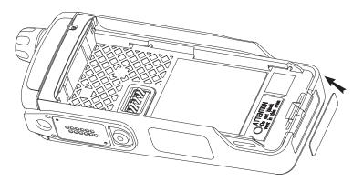
Figure 8-44. Assemble the Bottom Label
