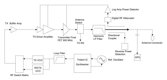
Figure 3-10. Transmitter (900 MHz) Block Diagram
