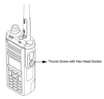
Figure 7-37. Securing the Cover
