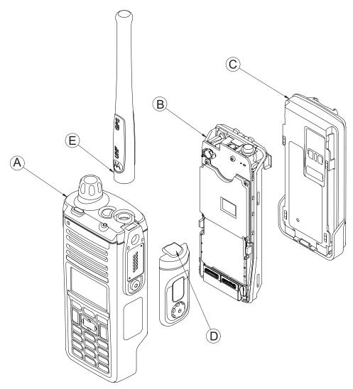
Figure 8-1. APX 2000/ APX 4000/ APX 4000Li Partial Exploded View
