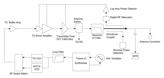
Figure 3-9. Transmitter (700/800 MHz) Block Diagram
