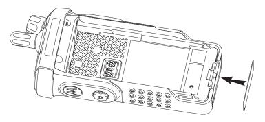
Figure 8-53. Assemble the Bottom Label
