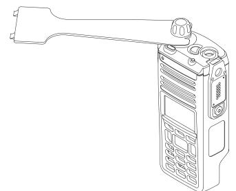
Figure 7-5. Removing the Multi Function Knob
