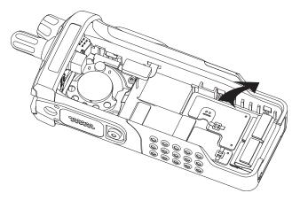
Figure 8-22. Remove the Keypad Board
