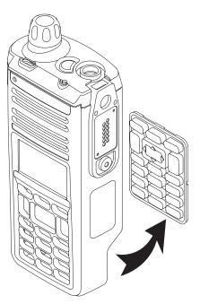
Figure 7-21. Remove the Keypad
