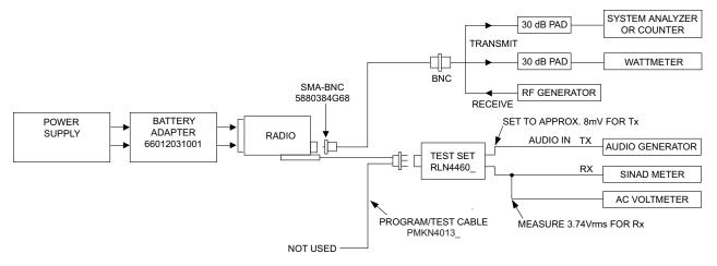
Figure 5-1. Performance Checks Test Setup
