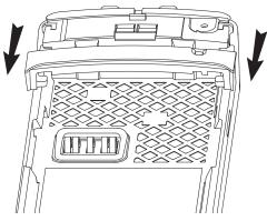
Figure 7-15. Remove the Shroud
