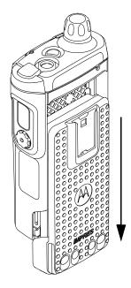
Figure 8-3. Removing the Battery
