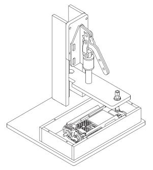
Figure 8-46. Attaching Vacuum Test Fixture
