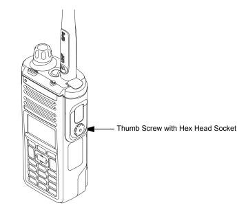
Figure 8-6. Removing the Thumb Screw
