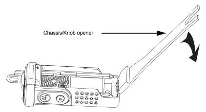
Figure 8-10. Disengage the Chassis
