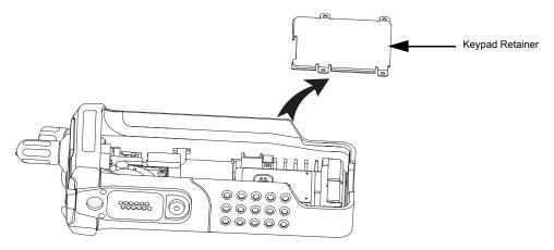
Figure 8-20. Remove the Keypad Retainer
