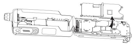
Figure 7-10. Remove the Secondary Shield Assembly
