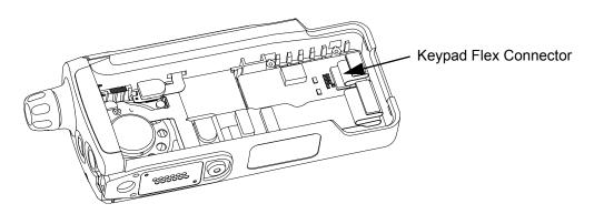
Figure 7-27. Rest the Front Kit Flex and plug in the Keypad Flex Connector
