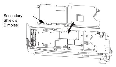
Figure 8-35. Assemble the Secondary Shield Assembly
