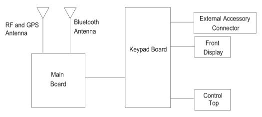
Figure 3-1. APX 2000/APX 4000/APX 4000Li Overall Block Diagram
