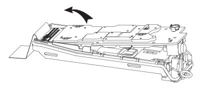
Figure 8-12. Lift up the Main Board from the Chassis
