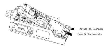
Figure 7-12. Unplug the connectors on the Front Kit Flex and Keypad Flex
