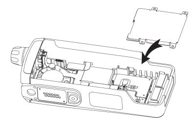
Figure 8-33. Place Keypad Retainer over the Keypad Board
