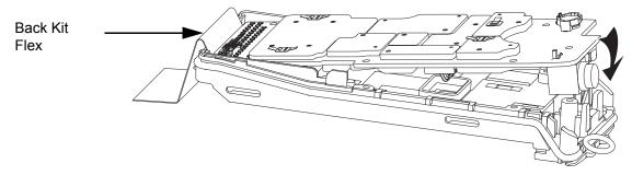
Figure 8-26. Assemble the RF Board
