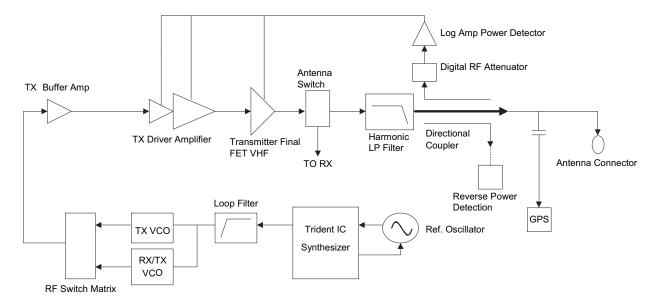
Figure 3-6. Transmitter (VHF) Block Diagram
