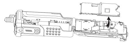
Figure 8-13. Remove the Secondary Shield Assembly
