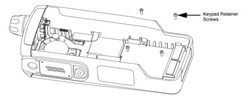
Figure 8-16. Remove the Keypad Retainer Screws
