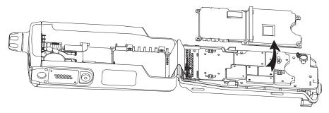
Figure 8-10. Remove the Secondary Shield Assembly
