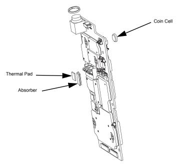
Figure 7-21. Serviceable Components – Main Board Assembly
