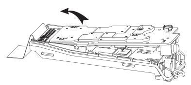
Figure 8-15. Lift up the Main Board from the Chassis
