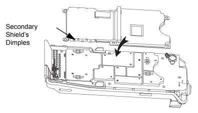
Figure 7-28. Assemble the Secondary Shield Assembly
