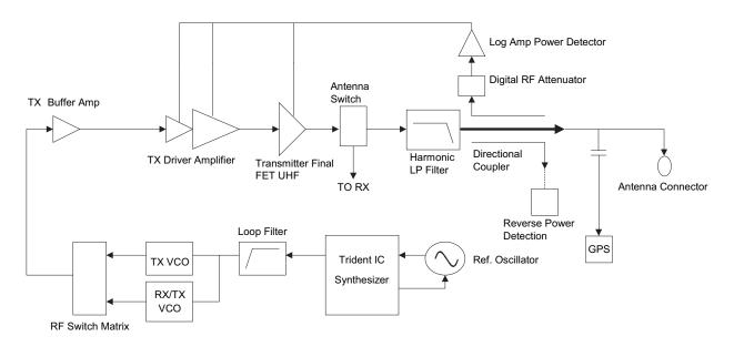
Figure 3-8. Transmitter (UHF1/UHF2) Block Diagram
