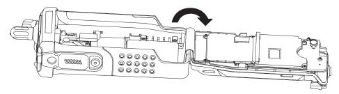
Figure 8-11. Remove the Chassis Assembly
