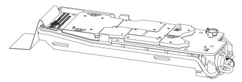
Figure 7-27. Assemble the Main O-Ring at Antenna Holder
