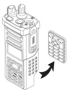
Figure 8-24. Remove the Keypad
