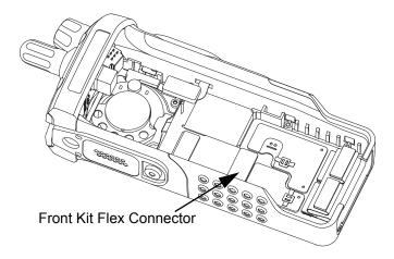
Figure 8-38. Plug in the Front Kit Flex Connector
