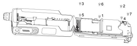
Figure 7-9. Remove the chassis screws
