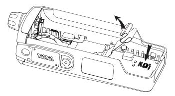
Figure 7-26. Plug in the Front Kit Flex Connector
