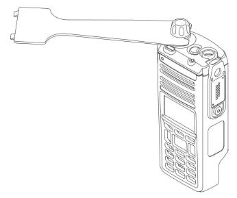
Figure 7-25. Servicing the Multi Function Knob
