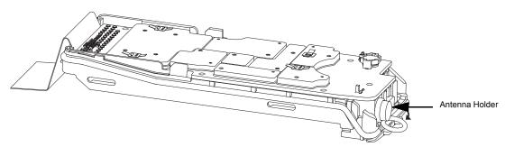
Figure 7-11. Remove the Main O-Ring at the antenna holder
