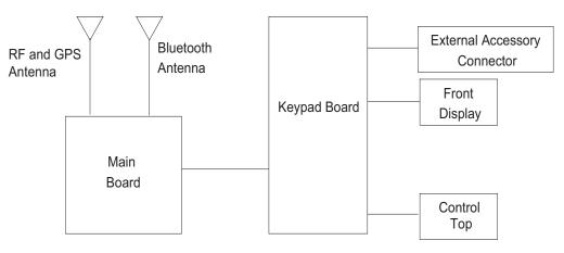
Figure 3-1. APX 1000 Overall Block Diagram
