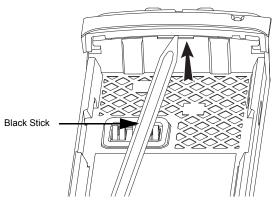
Figure 7-13. Disengage the Shroud
