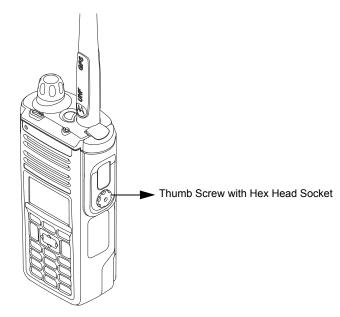
Figure 8-39. Securing the Cover
