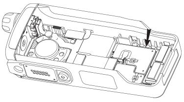
Figure 8-19. Remove the Keypad Board
