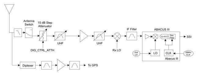
Figure 3-3. Receiver Block Diagram (UHF1/UHF2)
