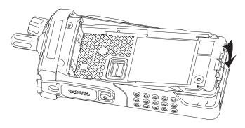
Figure 8-44. Assemble Back Kit and Front Kit together
