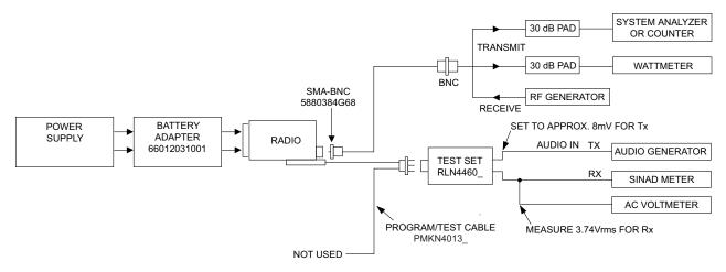
Figure 5-1. Performance Checks Test Setup
