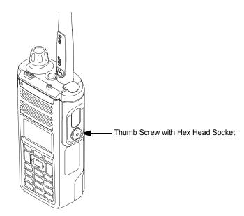
Figure 7-6. Removing the Thumb Screw
