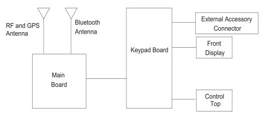
Figure 3-1. APX 2000/ APX 4000 (Two Knobs) Overall Block Diagram
