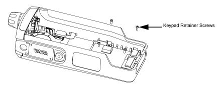
Figure 7-15. Remove the Keypad Retainer Screws
