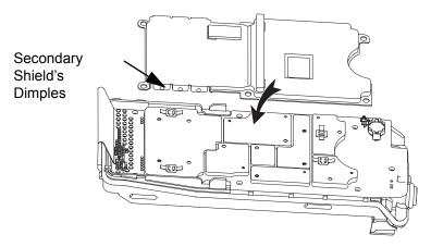
Figure 8-28. Assemble the Secondary Shield Assembly
