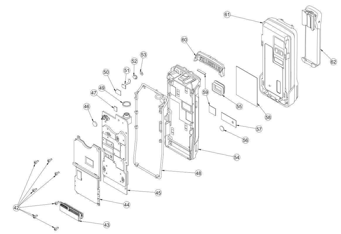
Figure 10-2. APX 2000/ APX 4000 (Two Knobs) Back Kit Exploded View
