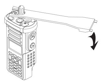
Figure 8-6. Removing the Channel Knob
