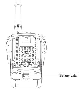
Figure 8-2. Lifting up the latch
