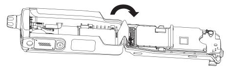
Figure 7-8. Remove the Chassis Assembly
