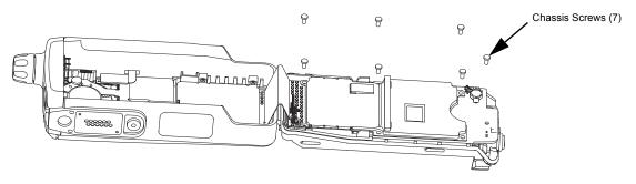
Figure 8-9. Remove the chassis screws
