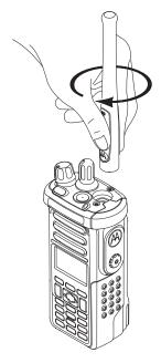
Figure 8-50. Attaching the Antenna
