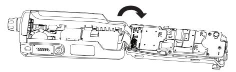
Figure 7-8. Remove the Chassis Assembly
