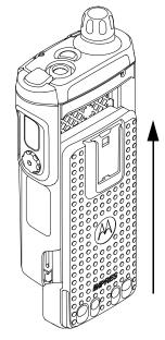
Figure 7-45. Attaching Battery – Slide into Position
