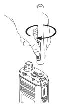
Figure 8-41. Attaching the Antenna
