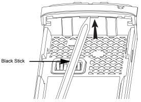
Figure 7-14. Disengage the Shroud
