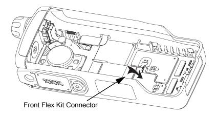
Figure 8-31. Plug in the Front Kit Flex Connector
