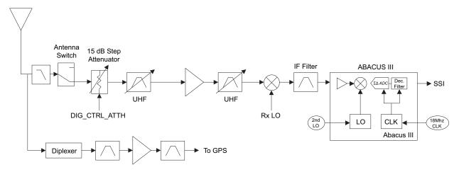
Figure 3-3. Receiver Block Diagram (UHF1/UHF2)
