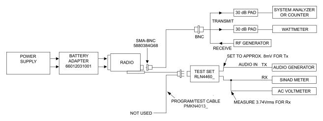
Figure 5-1. Performance Checks Test Setup
