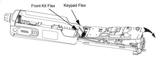
Figure 7-30. Assemble the RF Board
