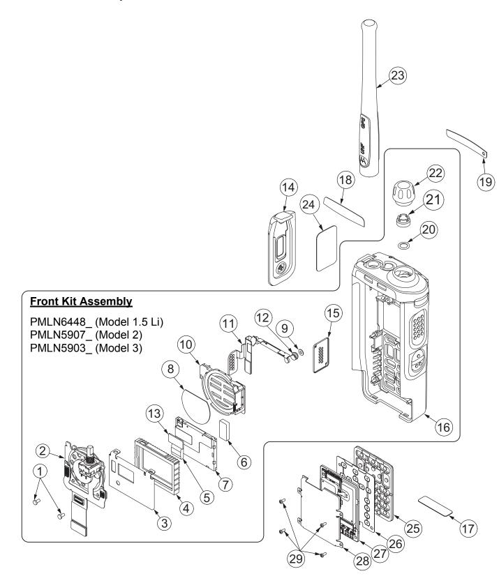
Figure 10-1. APX 2000/ APX 4000/ APX 4000Li Front Kit Exploded View
