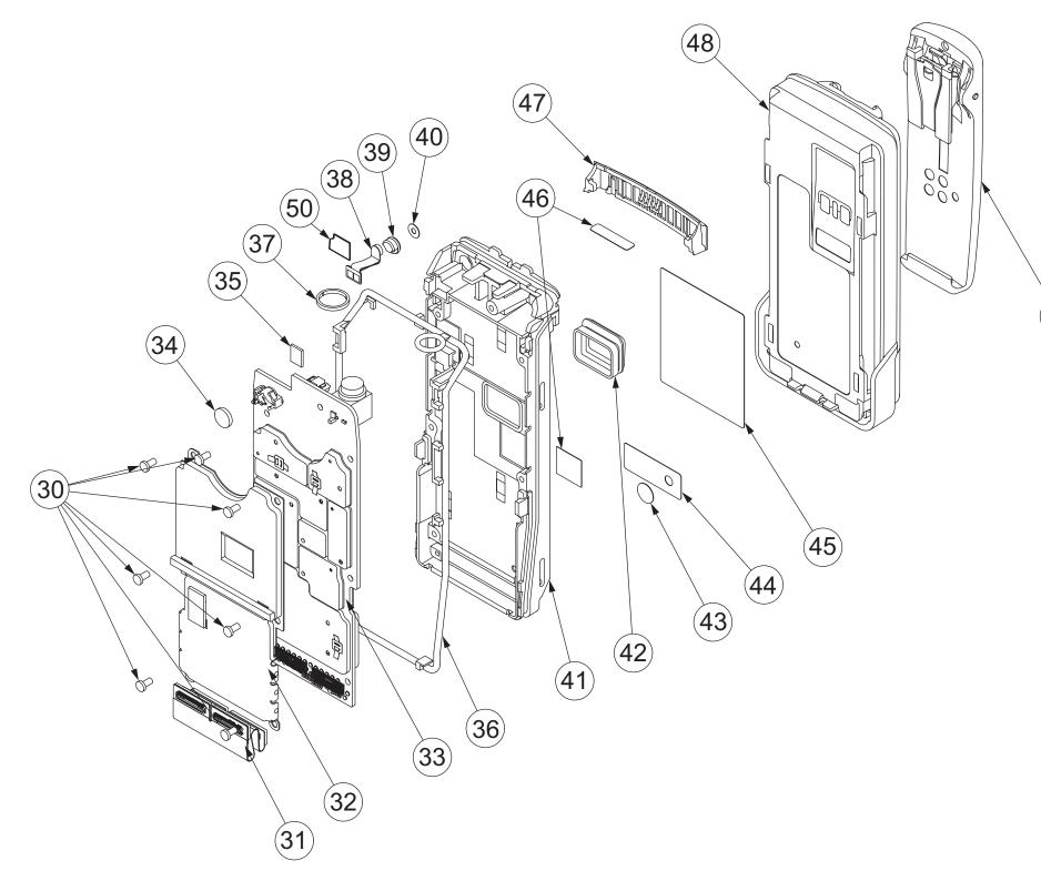
Figure 10-2. APX 2000/ APX 4000/ APX 4000Li Back Kit Exploded View
