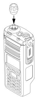
Figure 7-40. Reassemble the Multi Function Knob
