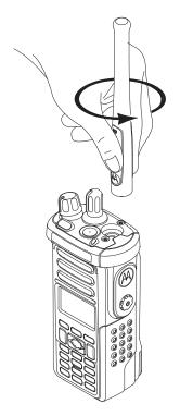
Figure 8-4. Removing the Antenna
