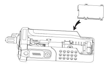
Figure 8-40. Place Keypad Retainer over the Keypad Board
