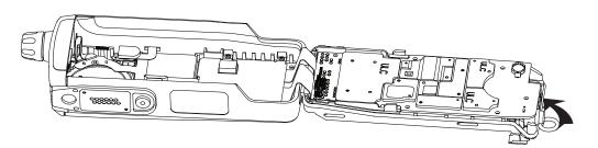
Figure 7-31. Assemble the Main O-Ring at Antenna Holder
