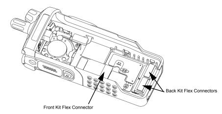
Figure 8-21. Unplug the Front Kit Flex and Back Kit Flex Connectors
