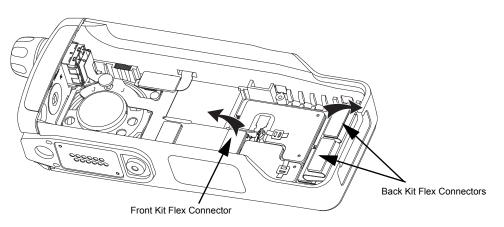
Figure 7-18. Unplug the Front Kit Flex and Back Kit Flex Connectors
