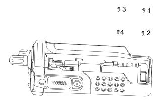
Figure 8-19. Remove the Keypad Retainer Screws
