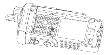
Figure 8-51. Assemble the Vacuum Port Seal
