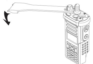
Figure 8-5. Removing the Volume Knob
