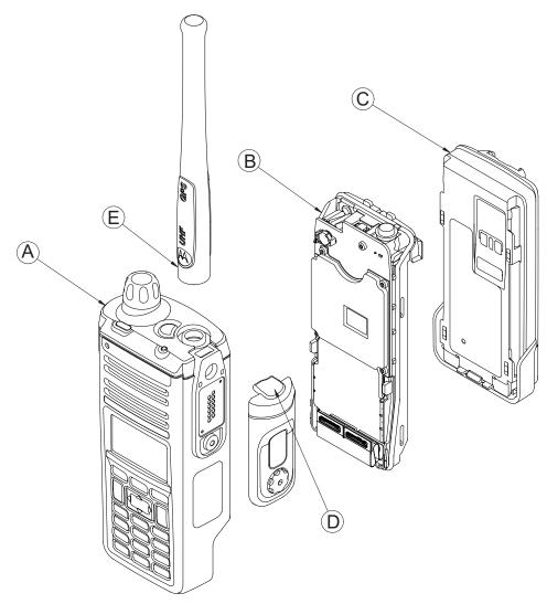
Figure 7-1. APX 1000 Partial Exploded View
