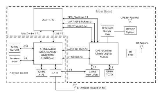
Figure 3-12. GPS/Bluetooth/Accelerometer Block Diagram
