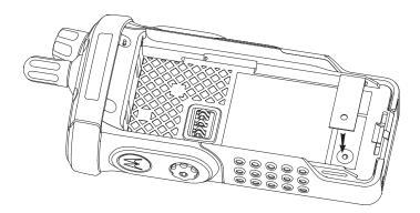
Figure 8-52. Assemble the Ventilation Label
