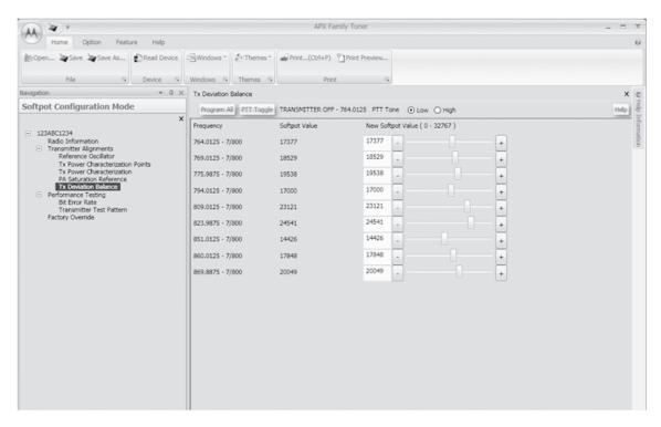
Figure 6-20. Transmit Deviation Balance Alignment Screen (700/800 MHz)
