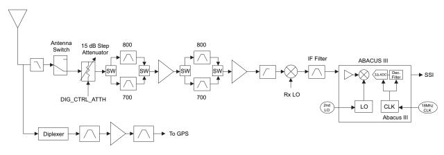
Figure 3-4. Receiver Block Diagram (700/800 MHz)
