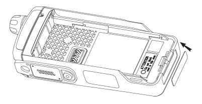
Figure 7-44. Assemble the Bottom Label
