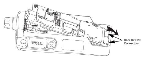
Figure 8-13. Unplug the Back Kit Flex connectors
