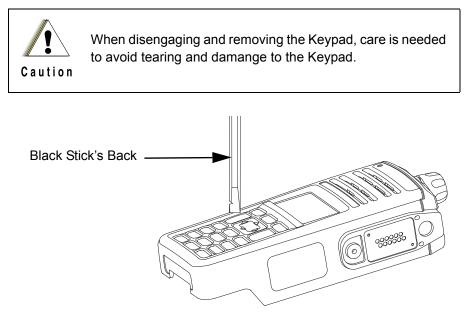
Figure 8-20. Disengage the Keypad
