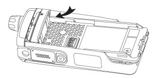
Figure 7-34. Slide chassis assembly into Front Housing
