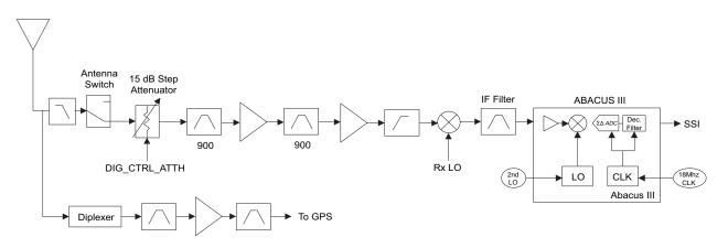
Figure 3-2. Receiver Block Diagram (900 MHz)
