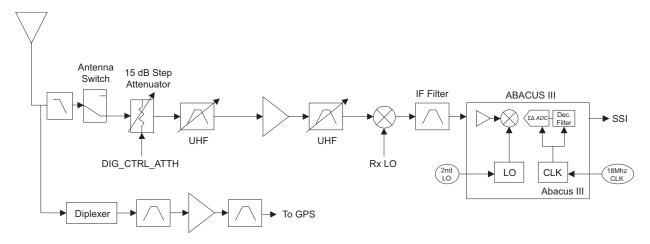
Figure 3-3. Receiver Block Diagram (UHF1/UHF2)
