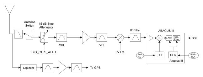
Figure 3-2. Receiver Block Diagram (VHF)
