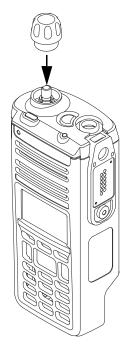
Figure 8-40. Reassemble the Multi Function Knob
