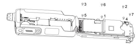
Figure 8-29. Torque in the Chassis Screws
