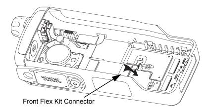
Figure 7-31. Plug in the Front Kit Flex Connector
