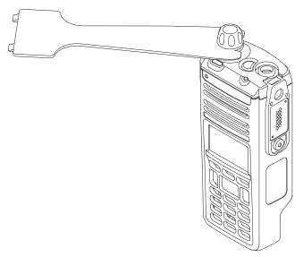
Figure 8-25. Servicing the Multi Function Knob
