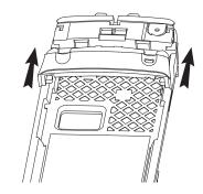
Figure 8-42. Assemble the Shroud
