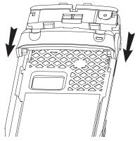
Figure 8-18. Remove the Shroud
