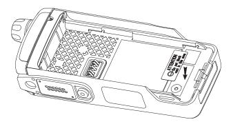
Figure 7-43. Assemble the Ventilation Label
