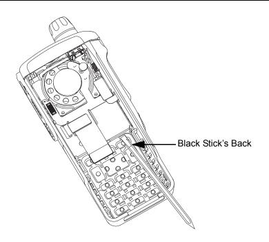
Figure 7-30. Assemble the Keypad
