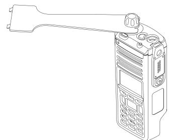
Figure 7-5. Removing the Multi Function Knob
